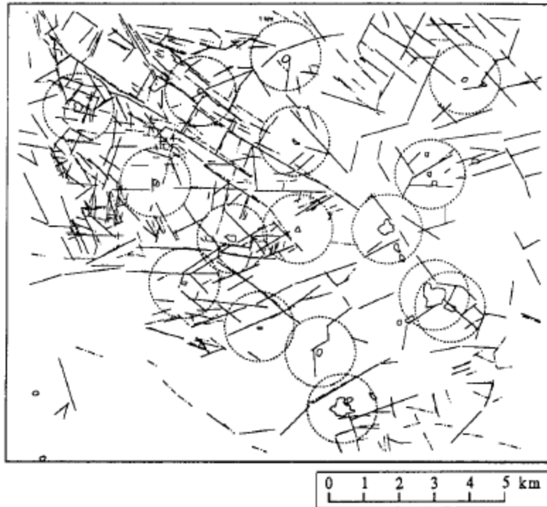
Fig. 2. The lineament study area, with lineaments (SPOT and Landsat TM) and circles with 1 km radius from the 16 village centers. The lineaments originate from the first mapping by a single interpreter.
