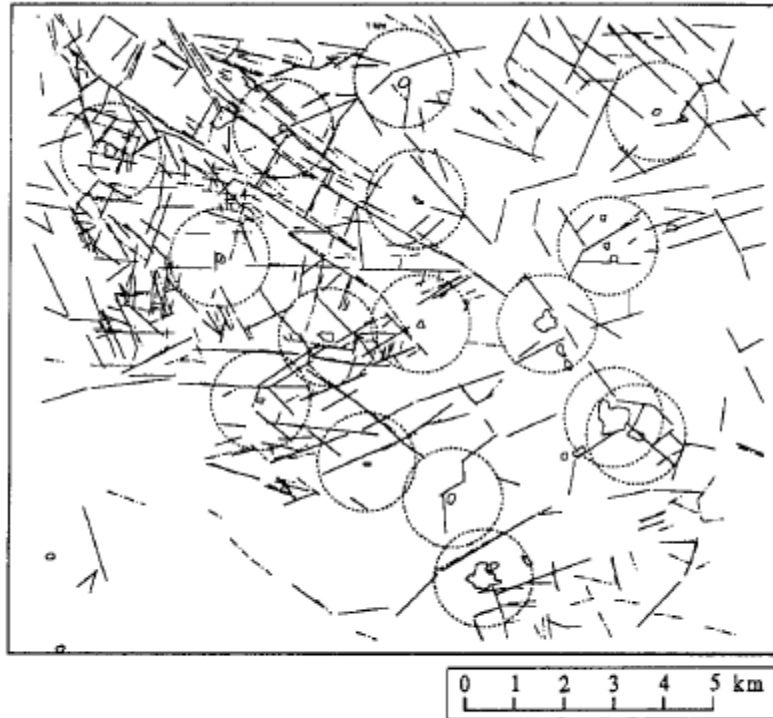
Fig. 2. The lineament study area, with lineaments (SPOT and Landsat TM) and circles with 1 km radius from the 16 village centers. The lineaments originate from the first mapping by a single interpreter.
